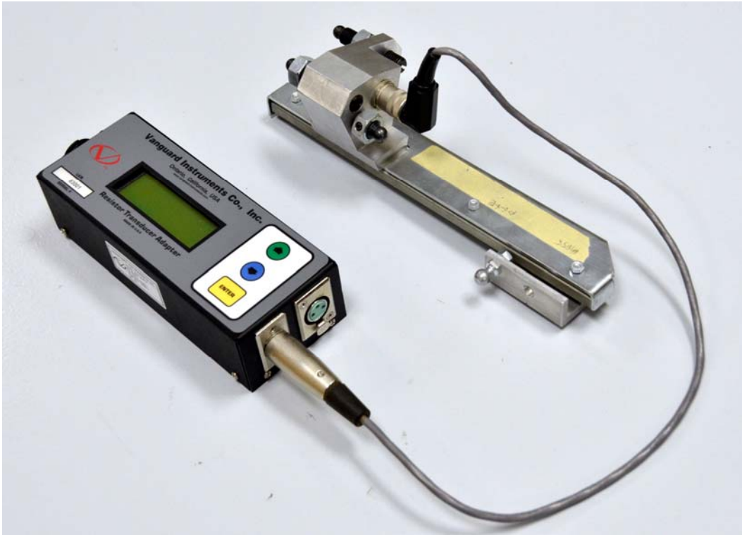
Figure 1. Typical Connection to ABB AHMB Transducer
