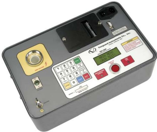
The VBT-80P is a microprocessor-based, portable 80 kV dc vacuum bottle tester. This light-weight, portable tester is designed for testing circuit-breaker vacuum bottles in the field and at the shop.
